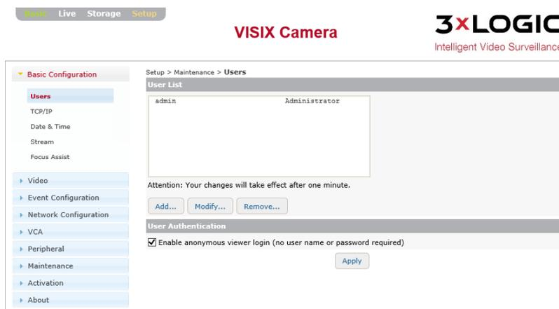
Figure 7-2: Setup Tab – Basic Configuration Menu – Users Settings
