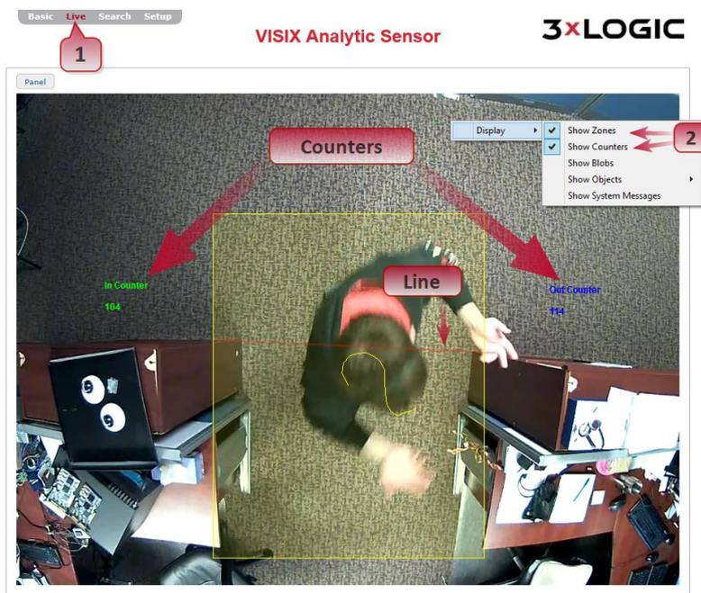
Figure 4-12: Example 1 Counting Line (Tripwire) Analytics Overlay
