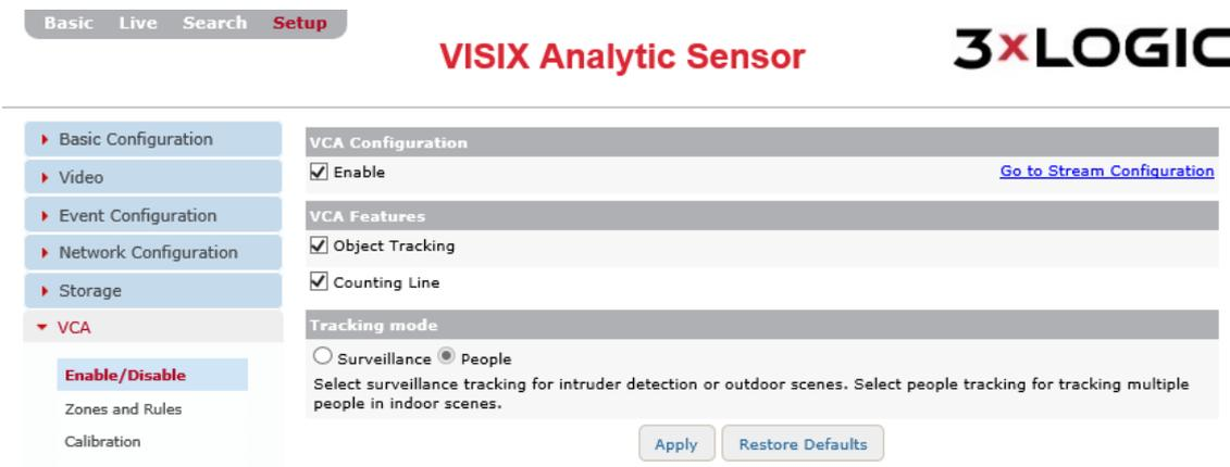
Figure 7-65: Setup Tab –VCA Menu –Enable/Disable Settings
