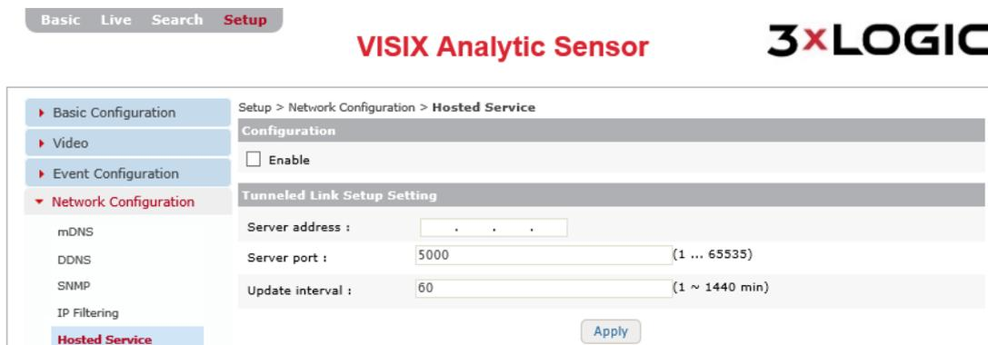
Figure 7-60: Setup Tab –Network Configuration Menu – Hosted Service Settings
