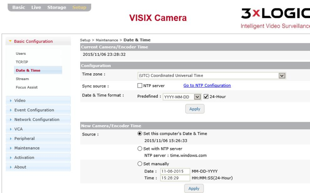
Figure 7-7: Setup Tab – Basic Configuration Menu – Date & Time Settings
