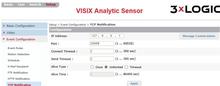
Figure 7-42: Setup Tab-Event Configuration Menu – TCP Notification Settings
