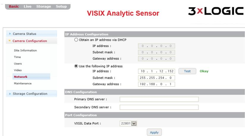
Figure 5-7: Basic Tab – Camera Configuration – Network Settings
