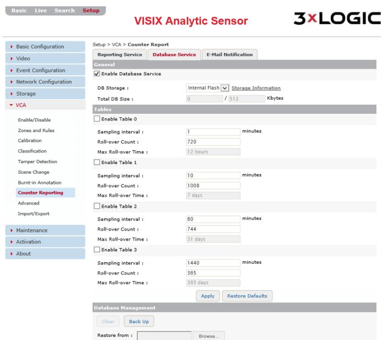
Figure 7-77: Setup Tab –VCA Menu –Counter Reporting Settings– Database Service Tab
