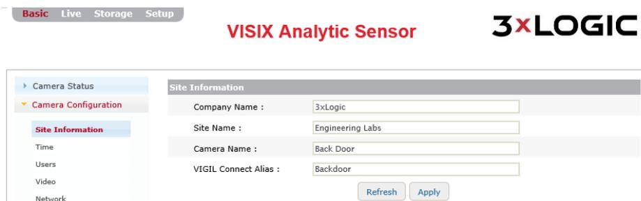
Figure 5-2: Basic Tab – Camera Configuration – Site Information Form
