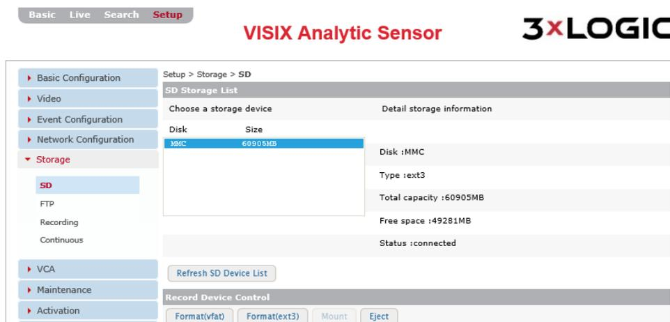
**Figure 7-61:** Setup Tab –Storage Menu – SD Settings
