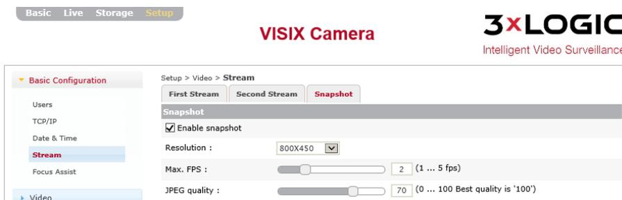
Figure 7-9: Setup Tab – Basic Configuration Menu –Snapshot Stream Settings
