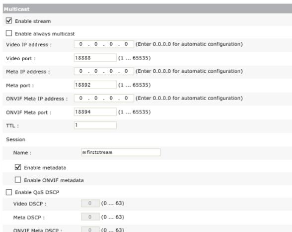
Figure 7-52: Setup Tab –Network Configuration Menu – RTSP/RTP Settings –Multicast Configuration
