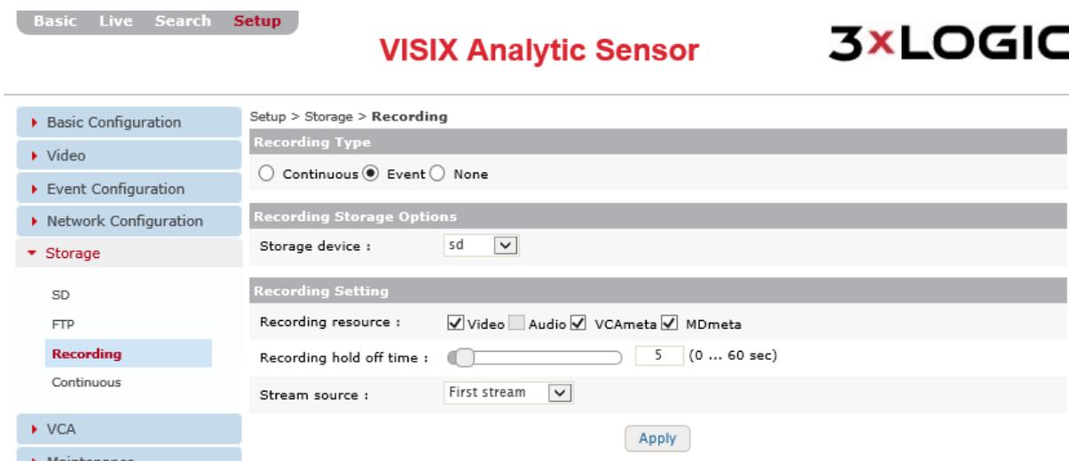
Figure 7-63: Setup Tab –Storage Menu –Recording Settings
