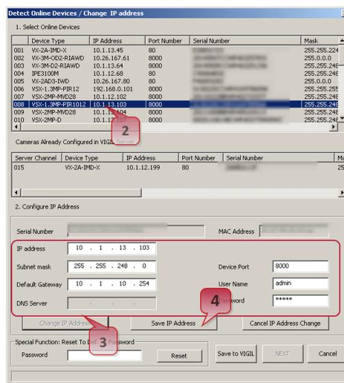
Figure 2-2: Identifying Device IP Address
