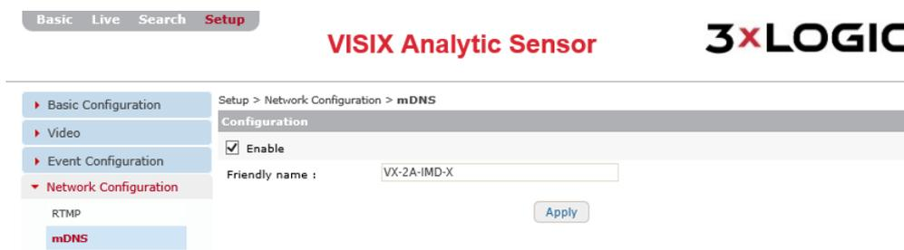
Figure 7-54: Setup Tab –Network Configuration Menu – mDNS Settings
