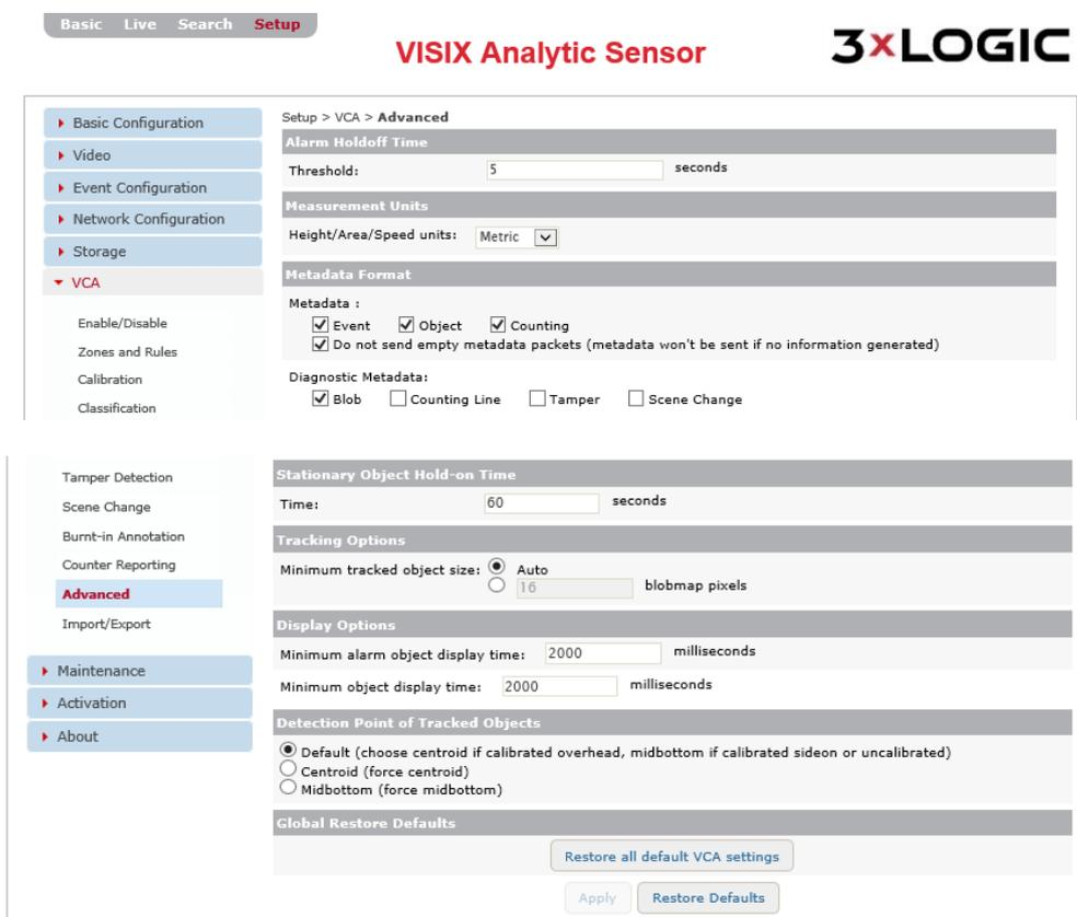
Figure 7-82: Setup Tab –VCA Menu –Advanced VCA Settings
