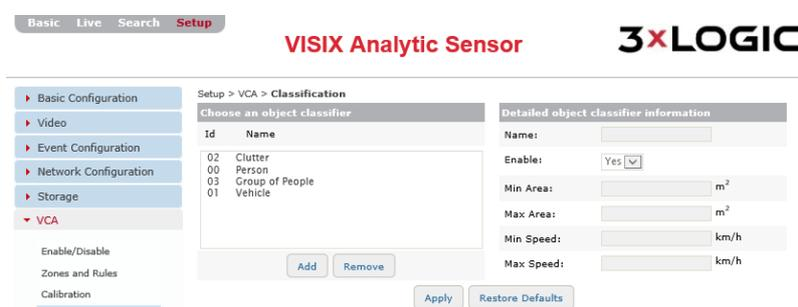
Figure 7-72: Setup Tab –VCA Menu –Classification Settings
