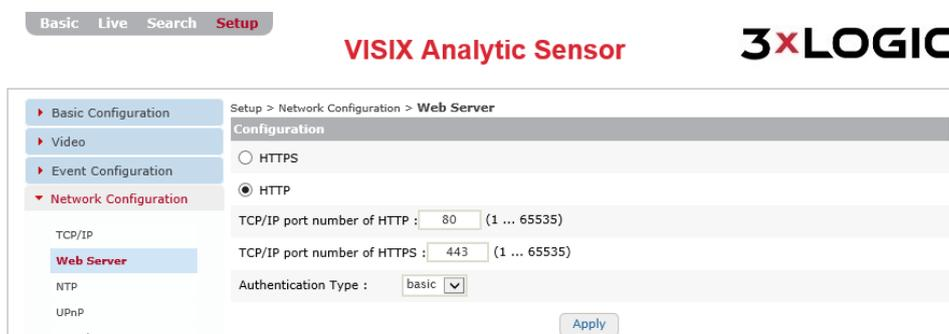
Figure 7-47: Setup Tab –Network Configuration Menu – Web Server Settings
