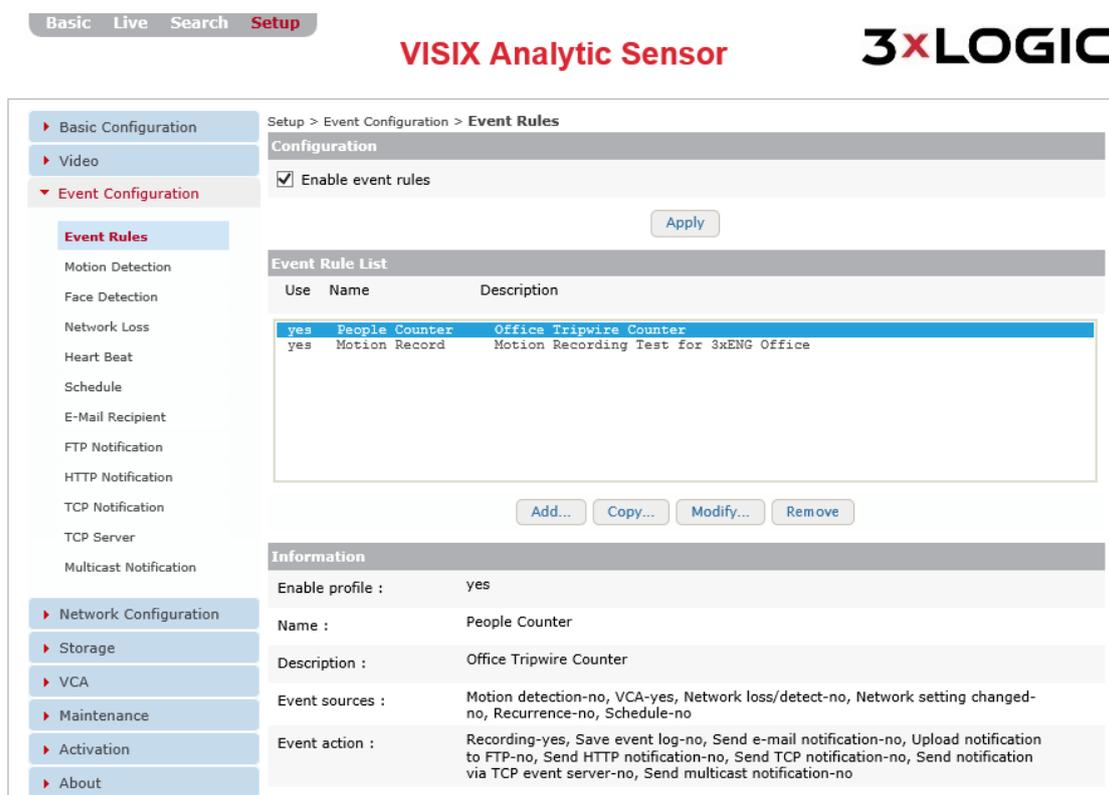
Figure 7-26: Setup Tab – Event Configuration – Event Rules Settings
