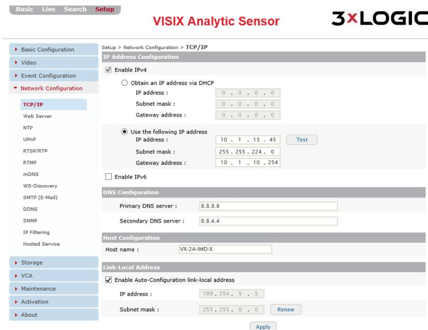
Figure 7-45: Setup Tab –Network Configuration Menu – TCP/IP Settings
