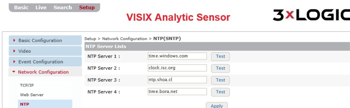
Figure 7-48: Setup Tab –Network Configuration Menu – NTP Settings
