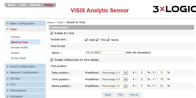
Figure 7-20: Setup Tab – Video Menu –Burnt-In Text Settings
