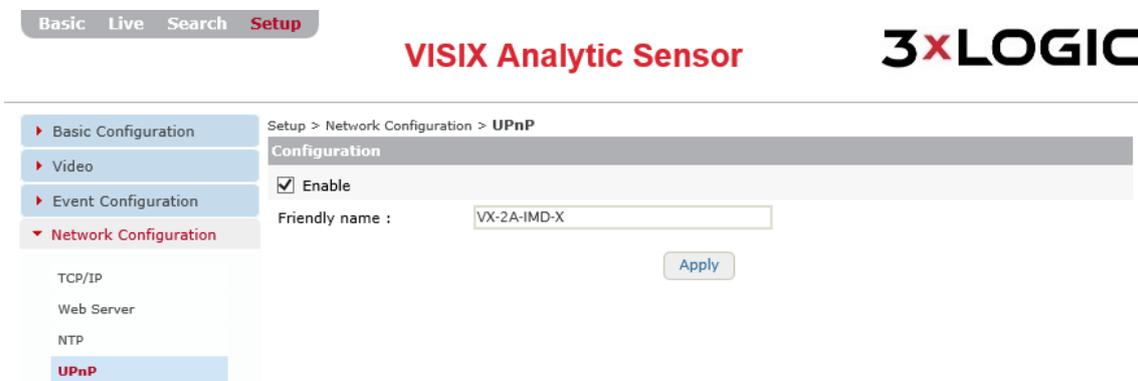
Figure 7-49: Setup Tab –Network Configuration Menu – UPnP Settings
