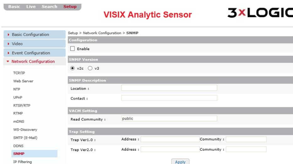
Figure 7-58: Setup Tab –Network Configuration Menu – SNMP Settings
