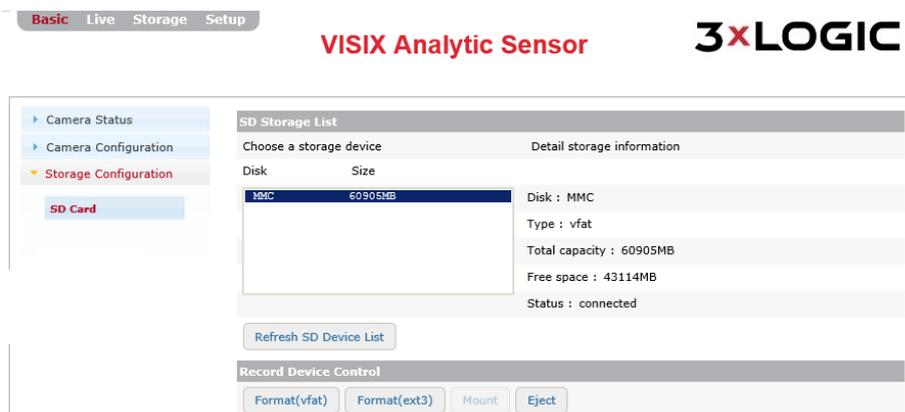
Figure 5-9: Basic Tab – Storage Configuration – SD Cards Settings
