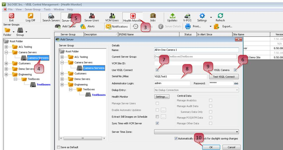
Figure 4-25: Adding an All-in-One Camera to VCM
