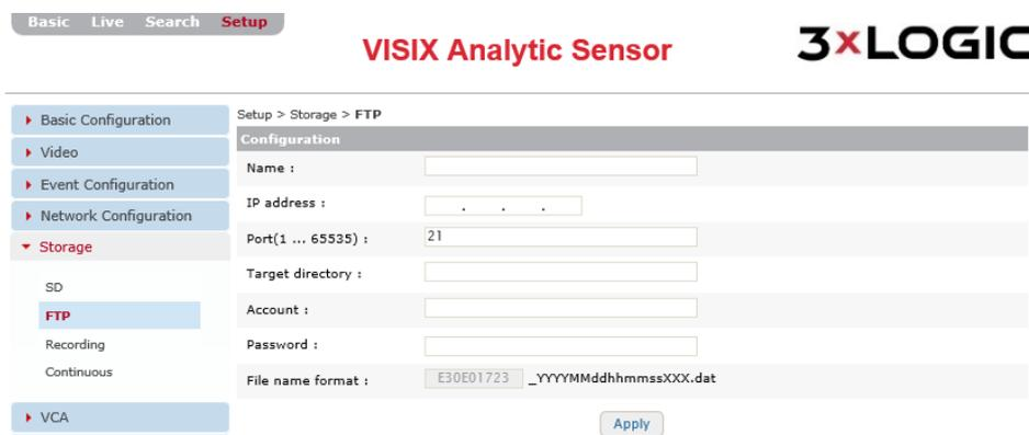
Figure 7-62: Setup Tab –Storage Menu –FTP Settings
