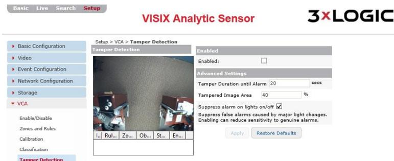
Figure 7-72: Setup Tab –VCA Menu –Tamper Detection Settings
