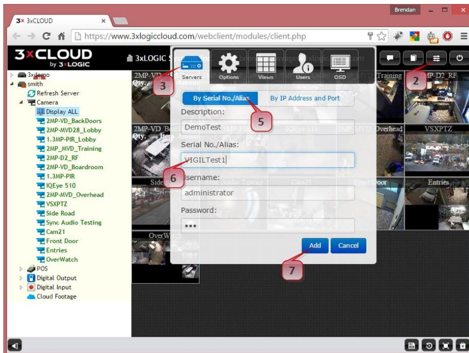
Figure 4-27: Adding an All-in-One Camera to a 3xCLOUD Account
