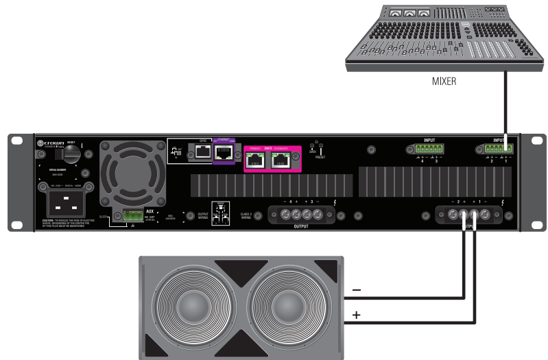
Figure 23: System wiring in Bridge Mono mode
