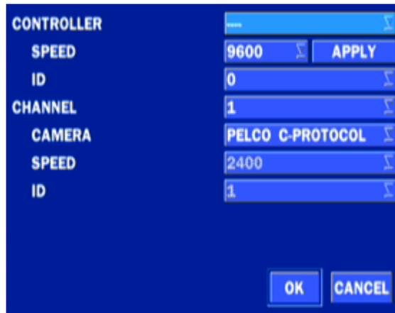
**Figure 4.4.5. PTZ Control Setup Screen**
