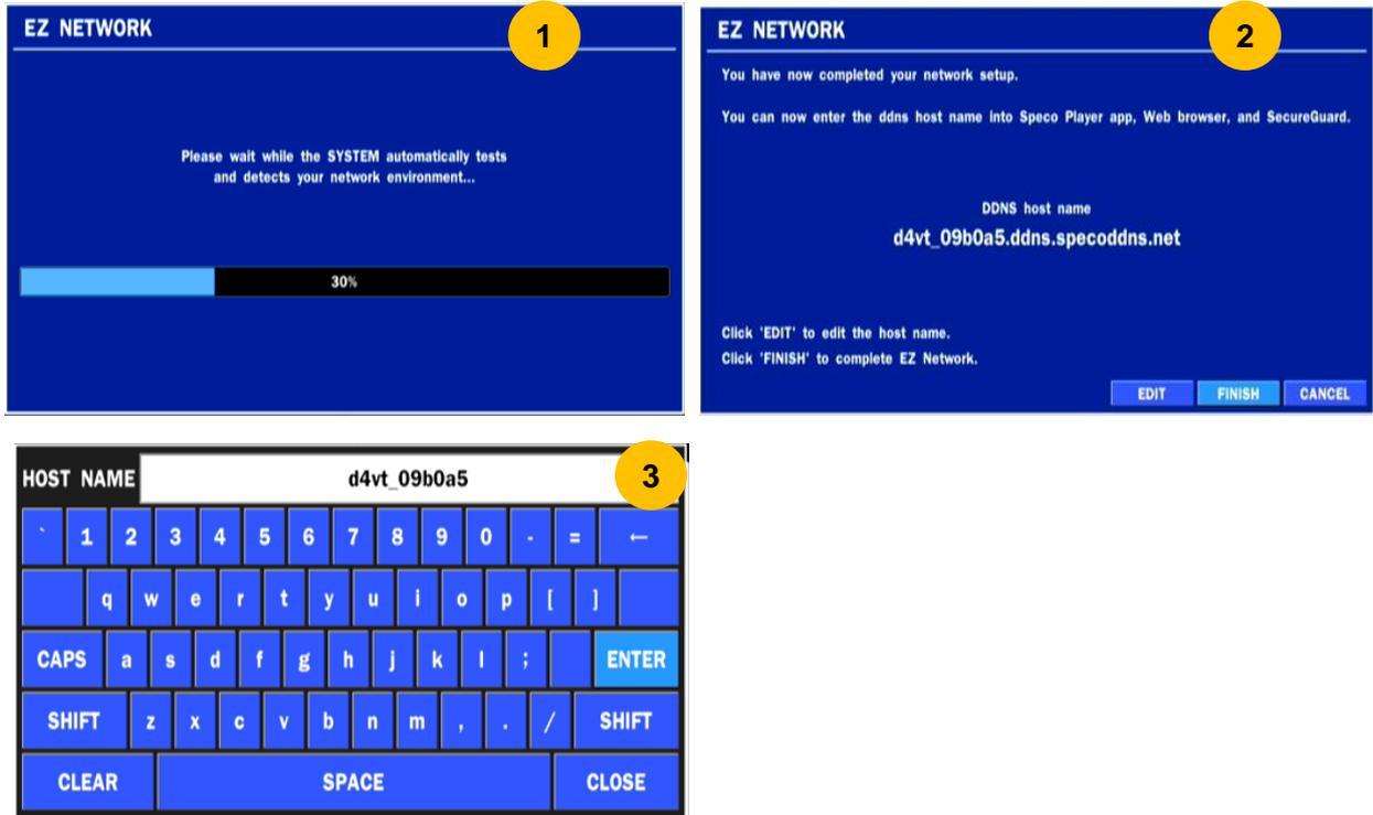
**Figure 2.4.2. EZ NETWORK Setup Procedure**
