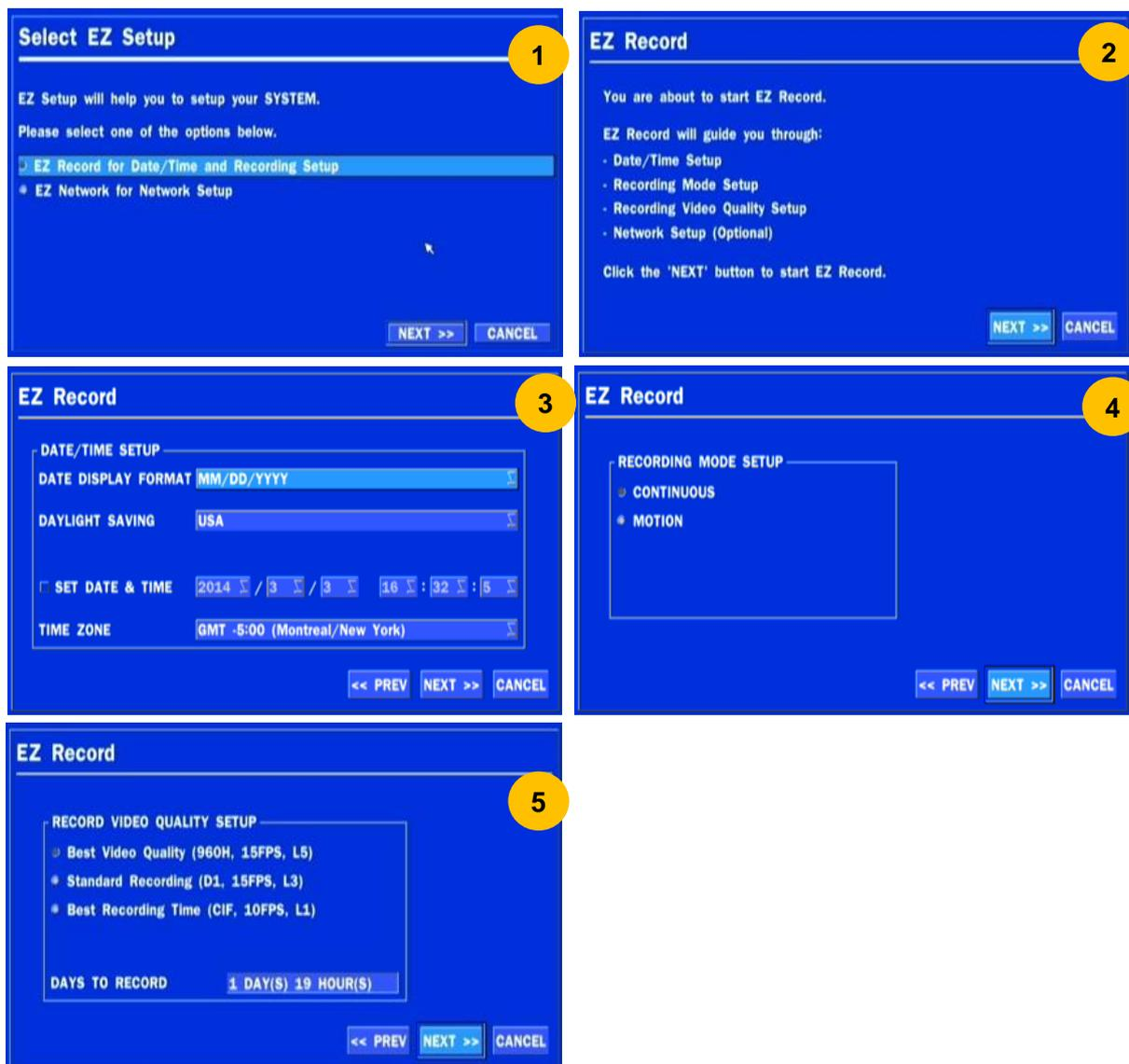
Figure 2.4.1. EZ Record Setup Procedure
