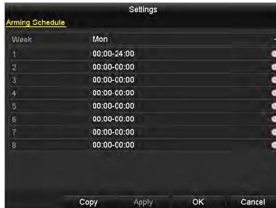
Figure 8. 24 Set Arming Schedule of Alarm Output
