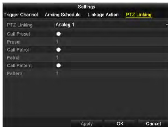
Figure 8. 8 Set PTZ Linking of Alarm Input
