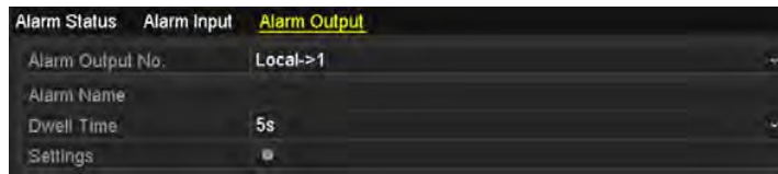
Figure 8. 23 Alarm Output Settings Interface
