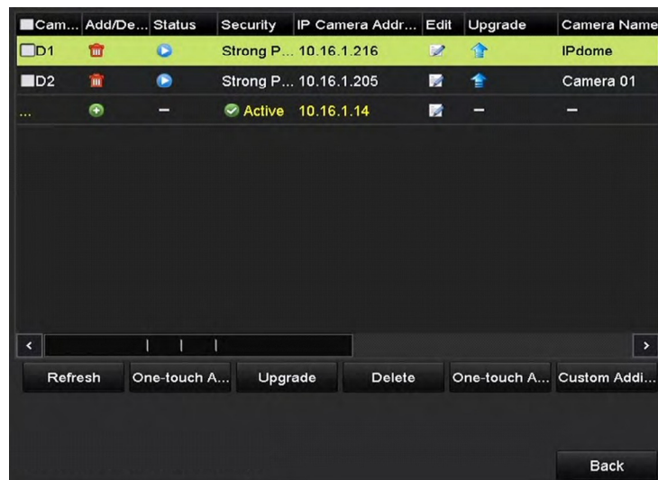
Figure 2. 21 Successfully Added IP Cameras
