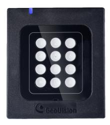
GV-RK1352 is a card reader with keypad, designed to recognize PIN codes, access control cards or both. Featured with the Wiegand and RS-485 interfaces, GV-RK1352 can be connected to any standard access control systems. GV-RK1352 comes with a weather sealed and IP66 compliant housing for outdoor use.
