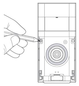
(If you're installing on wood, skip this step.) Use four of the provided Short Mounting Screws to secure your Ring Doorbell directly to the wall. Secure your Ring Doorbell.
