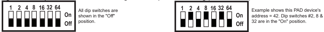
Figure 2. Examples of PAD Device Showing Default Dip Switch Setting (Unaddressed) & Addressed PAD Device
