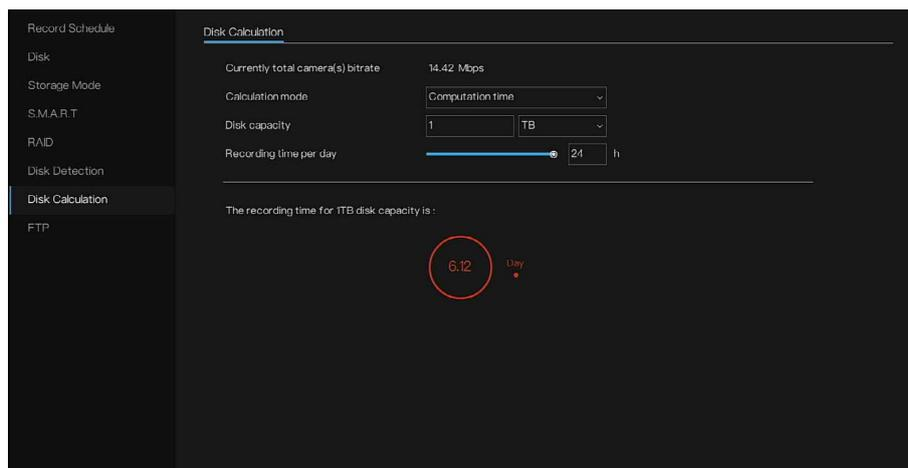
*Note: The computation is based on the currently online cameras bitrate (includes main stream and sub stream).*
