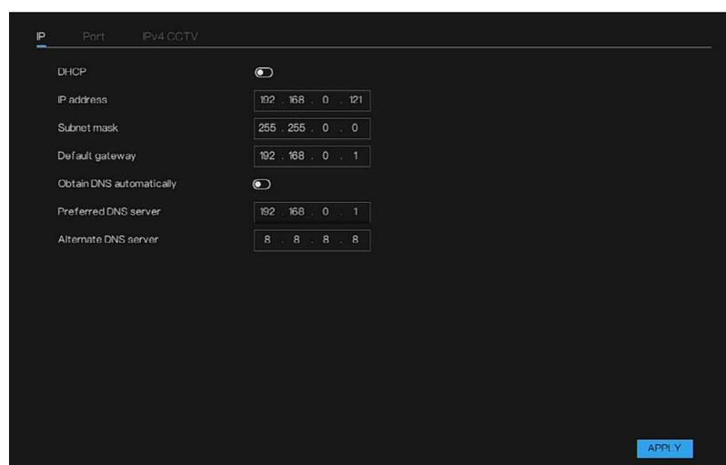
2. Enable DHCP and the router can distribute the IP automatically.
