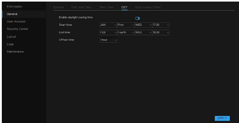
3. Configure the start time and end time for the DST. For the start time, the time will delay one hour (or half hours, it depends on the local rules).
