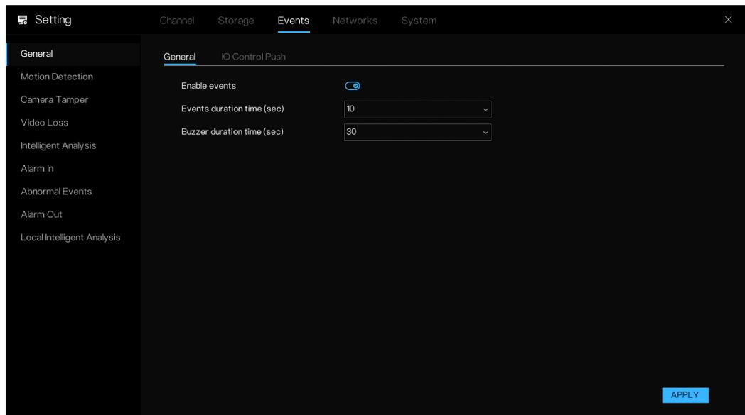
2. Enable alarm, set Alarm duration time(sec) and Buzzer duration time(sec).
