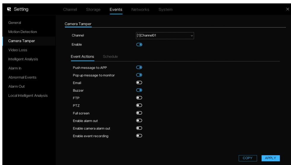
2. To configure the settings for the tampering detection parameters, refer to [Motion Detection](#).
