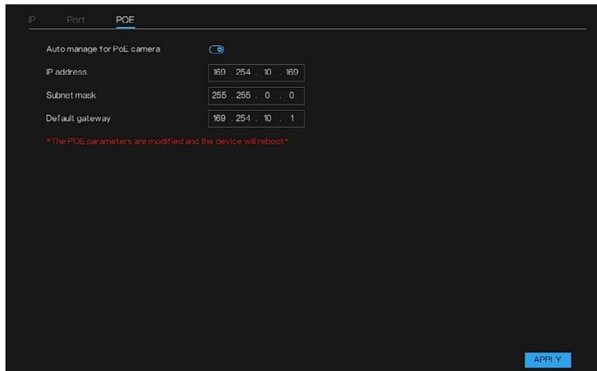
2. The default Auto manage for PoE camera is open. Users can set the PoE camera IP parameters manually.
