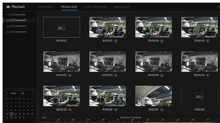
2. Select a camera in the camera list on the left side of the picture grid screen. Videos shot by the camera in the earliest time range on the current day are displayed as thumbnails in the window on the right side.
