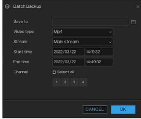
choose the path to save, video type (MP4 or AVI), stream (Main stream or sub stream); Set the start time and end time; choose channels; click OK to download. The result shows at Backup List interface.                                                                                                                        |
