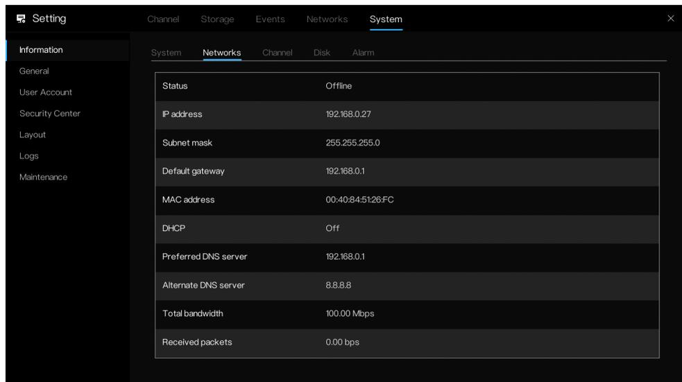
The screenshot shows the 'Setting' application with the 'System' tab selected. The 'Networks' sub-tab is active, displaying a table of network configuration details.
