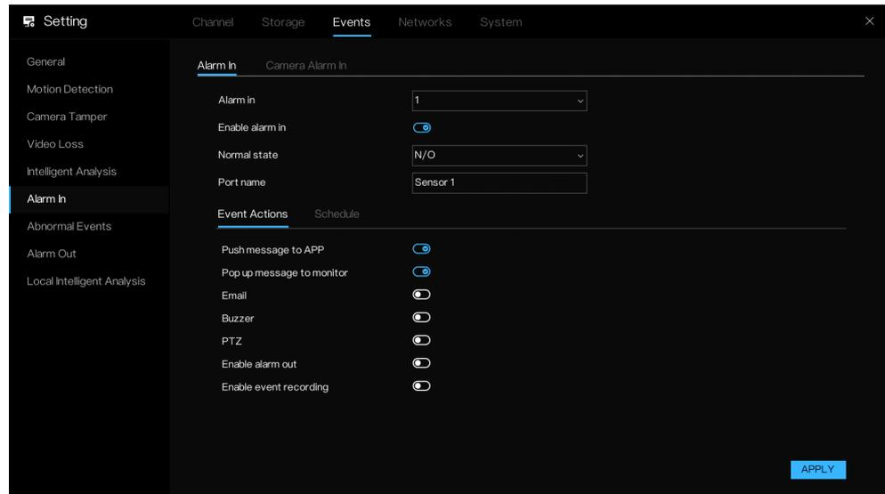
2. Set Alarm-in Port channel number and then select the enable check box to enable the function.
