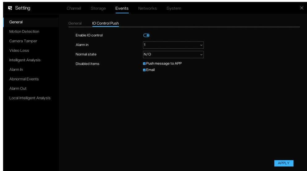
2. Enable IO Control Push, choose the Alarm in from drop-down list.
