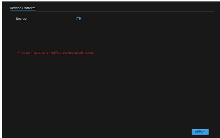
2. Encrypt the device, when you add the NVR to HSV platform, choose the private protocol(encrypt).
