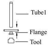
2. Use the tool to fix the flange and the tube1 (You can also directly install Tube2 if you don't want to install Tube1).
