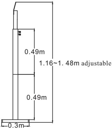
The adjustable range of the bracket without Tube1 is from 0.67m to 0.99m.
