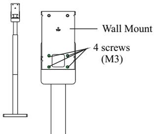
5. Install the wall mount onto the bracket and then fix it with 4 screws.
