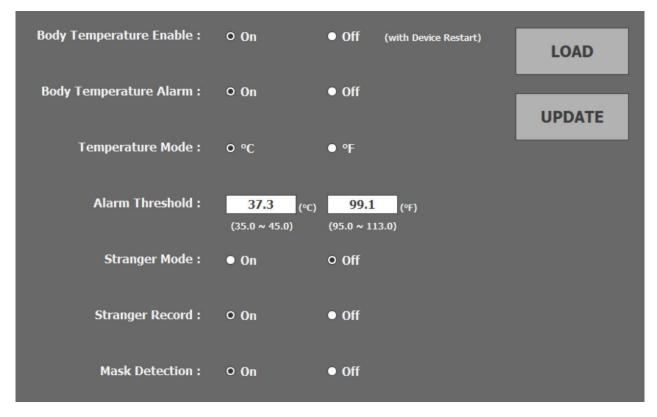
**-Temperature** Default setting is On, and when changed to Off, the device does not measure Temp. **measurement mode:** (only the facial recognition function operates). Device reboots when setting is changed.
