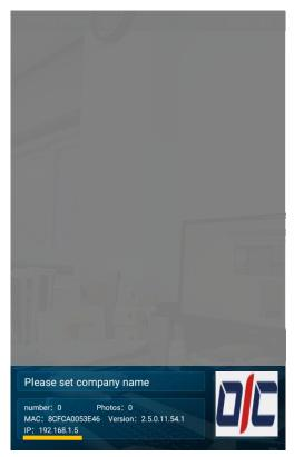
② Check the IP address of the control unit (Final version of OPASS app is 2.5.0.11.54.5) In the photo above, the device's IP address is 192.168.1.5.
