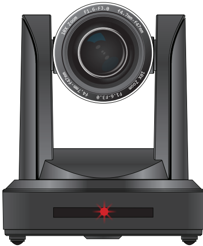
Flashing red LED during initialization
