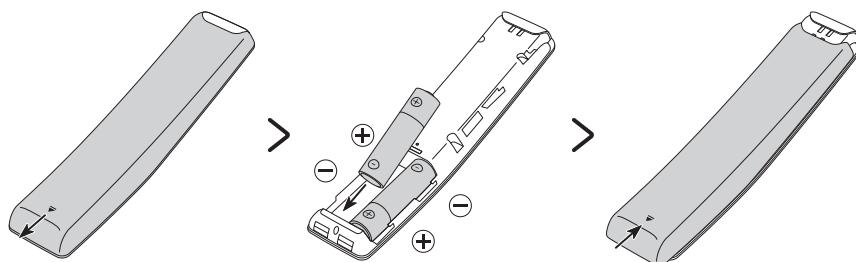
To install the batteries (1.5V AA type), push the rear cover open in the direction of the arrow at the bottom of the illustration, and then insert the batteries as shown in the figure. Make sure that the positive and negative ends are facing in the correct direction. Close the rear cover as shown.
