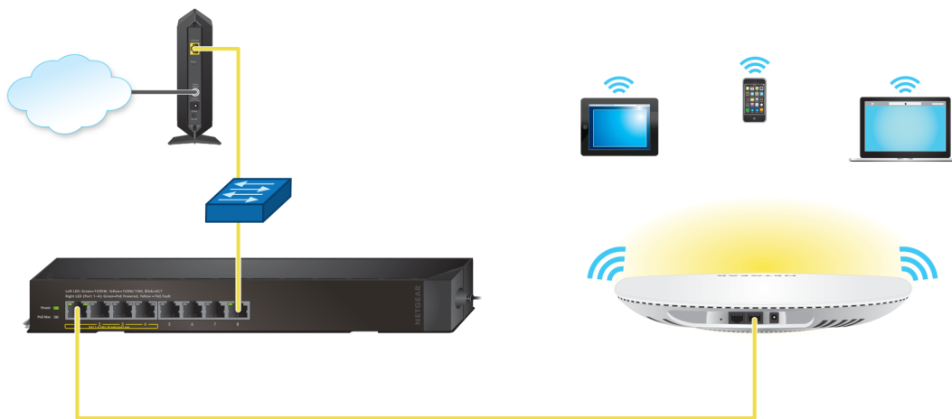
Figure 4. Set up the access point with a PoE+ connection to your network
