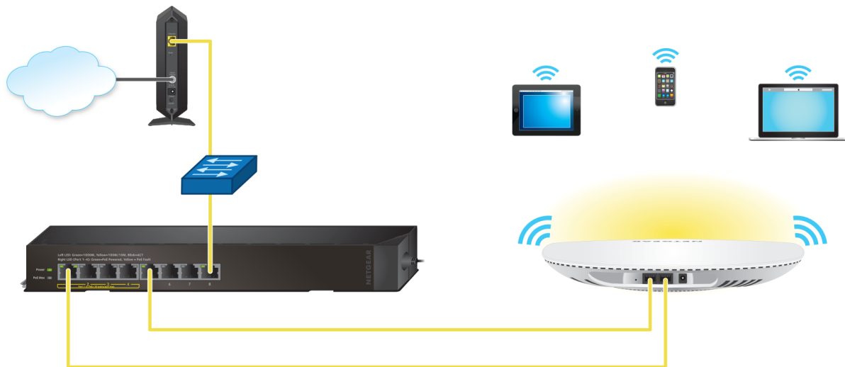
Figure 7. Link aggregation connection
