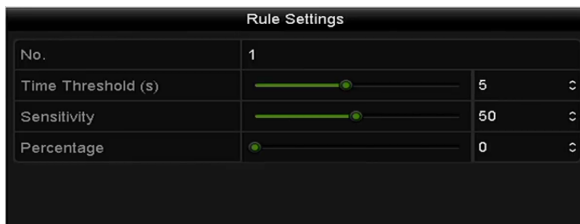
Figure 9-5 Set Intrusion Crossing Detection Rules
