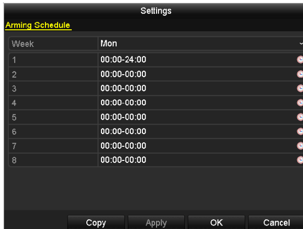
Figure 8-17 Set Arming Schedule of Alarm Output
