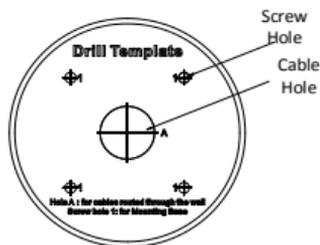
Figure 2. 28 The Drill Template
