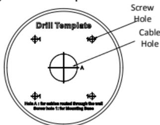
Figure 2. 24 The Drill Template
