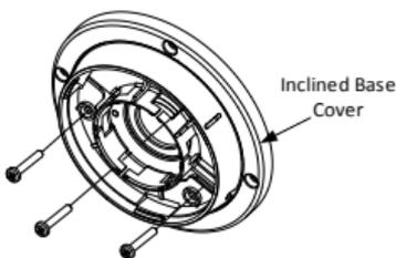
Figure 2. 29 Install Turret Camera's Mounting Base
