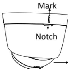
Figure 2. 19 Disassemble the Camera
