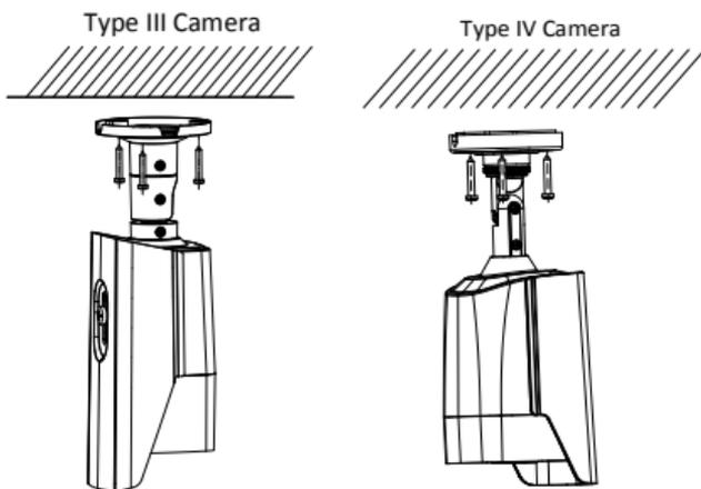
Figure 2.14 Fix the Camera to the Ceiling
