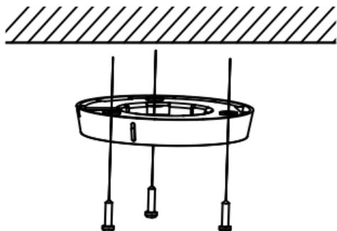
Figure 2. 21 Attach the Mounting Base to the Ceiling
