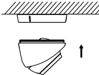
Figure 2. 22 Secure the Camera with Mounting Base
