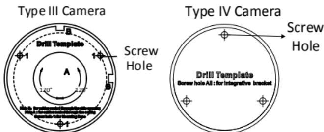
Figure 2.13 The Drill Template
