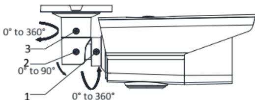
Figure 2. 16 3-Axis Adjustment
