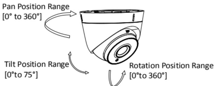
Figure 2. 23 3-axis Adjustment
