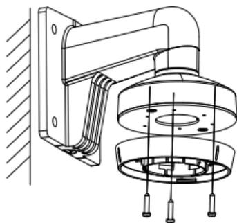
Figure 2. 27 Attach the Mounting Base to the Bracket
