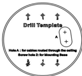
Figure 2. 1 The Drill Template
