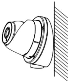
Figure 2. 31 Fix the Camera to the Inclined Base
