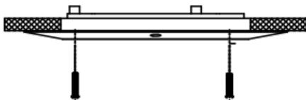
Figure 2. 7 Install the In-Ceiling Mounting Bracket
