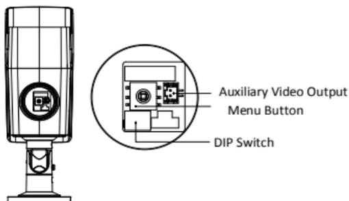
Figure 2. 15 Internal Interface and Button
