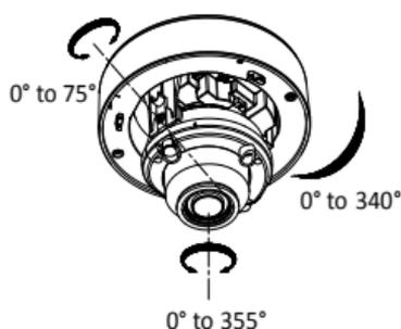
Figure 2. 4 3-Axis Adjustment
