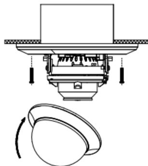
Figure 2. 10 Fix the Camera to the Junction Box
