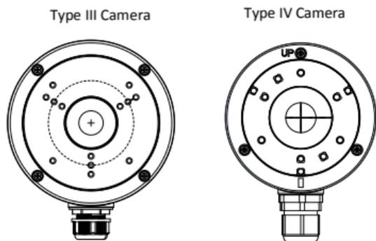
Figure 2. 17 Install the Junction Box
