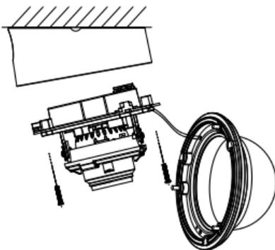
Figure 2. 12 Fix the Camera to the Base
