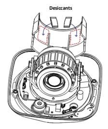
Step 4: Carefully tear open the vacuum-packed aluminum desiccant bag along the slit on one edge. Remove the desiccant. Remove the paper backing of the double-sided tape on one side of the desiccant. Firmly place the desiccant on the spot as illustrated.
