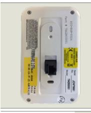
An E-Plex Gateway provides two-way communication from an E-Plex Lock to Keyscan Aurora software. A Gateway communicates to Aurora by a direct connection to a USB (non-network) or TCP/IP network. A Router acts as a repeater, extending the radio frequency (RF) communication between the Gateway and E-Plex Locks.
