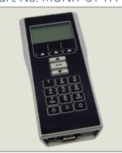
The M-Unit is a diagnostic and configuration data transfer tool designed to be used with E-Plex locks. It allows programming of offline E-Plex locks by gathering data from Aurora/LUNA software and transferring it the lock. It can also transfer audit trails and be used as a site survey tool for efficient placements for E-Plex wireless lock systems.
