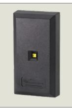
Farpointe Data mullion mount Indala format proximity surface mount reader. Wiegand output. Reads the Keyscan 125 kHz 36-bit Indala format. A HID PX-603 replacement reader. Black. 18" (457.2 mm) – 9 conductor shielded cable pigtail. Two-piece design with snap-on cover to hide mounting screws. Weight is 3 oz (85 g). Product Listings: UL294, FCC, IC. Warranty: Limited
