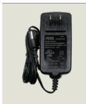
The PS1225 is a replacement 12VDC plug-in switching transformer for the SDACSKT (SDAC Kit). Plugs into standard 120 Vac outlet and provides up to 2.5 amps. Has 60" of 18 Gauge cable for mounting close to SDAC control. Has 2.1 mm barrel power connector. Center positive. For replacement of transformer provided in the SDACSKT. C/UL/US Listed Black Colour
