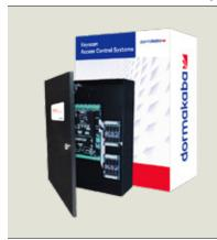
The Keyscan CA8500M is a network appliance-based access control unit that gives you unmatched flexibility for new installations or revitalizing aged or failing access control systems. The CA8500M is a package that includes 1 CA8500B ACU board, 2-OCB8 relay boards, 1-DPS-15 power supply, and 1-black metal enclosure with lock and tamper switch. This unit is special order hardware programmed for up to 90,000 credentials. It functions only with Aurora software.
