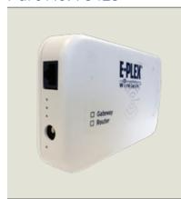
An E-Plex Gateway provides two-way communication from an E-Plex Lock to Keyscan Aurora software. A Gateway communicates to Aurora by a direct connection to a USB (non-network) or TCP/IP network. A Router acts as a repeater, extending the radio frequency (RF) communication between the Gateway and E-Plex Locks.
