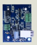
Networking a Keyscan access control unit is made easy by using the Keyscan NETCOM2 TCP/IP module. Allows maximum system design options. NETCOM2 is designed as an off-board adapter that can be installed within the metal enclosure and connected to the CIM to establish network communication using CAN Bus communication network. You can also connect to ACU board in other applications.
