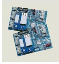
The Keyscan CIM-Link is a TCP/IP companion module, which incorporates multiple CIM CAN Bus communication loops into a single global infrastructure via LAN/WAN network. It maximizes system design options and promotes greater global communication flexibility across your facility. CIM-Link expands ACU to ACU functionality to multiple independent CAN Bus global networks.
