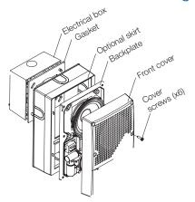
WG4 signals are rated for outdoor use and are suitable for indoor or outdoor applications on walls or ceilings. For surface-mounting in outdoor or wet applications, appliances must be mounted to an Edwards 449 electrical box. In dry conditions, they are compatible with standard 4-inch by 1½-inch deep electrical boxes. When using the optional
