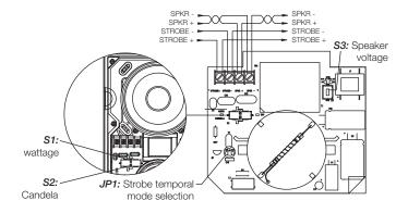
Genesis speaker-strobes may also be configured for temporal flash. This power-saving feature is intended for private mode signaling only. To set the device for temporal flash, snip the jumper at **JP1**.
