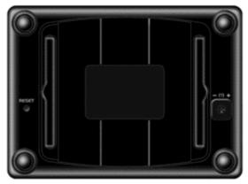
**Reset Button**: The Reset button is located on the bottom of the unit, and requires a stylus, or paper clip to press the button. Pressing the Reset button will cycle the MRX-4IR's power. (Unplugging the MRX-4IR's power cable and then plugging it back in, also performs the same function.)
