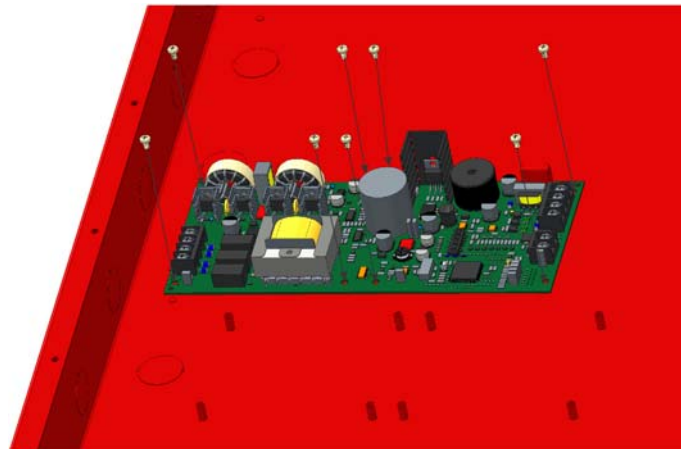
Figure 4.22 EVS-INT50W in FACP Cabinet
