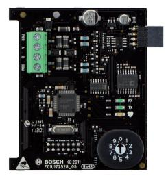
The B820 Inovonics Interface Module is a fully supervised, addressable SDI2 bus device that allows communication between Bosch control panels and an Inovonics EN4200 EchoStream Serial Receiver with EchoStream Wireless transmitters.
