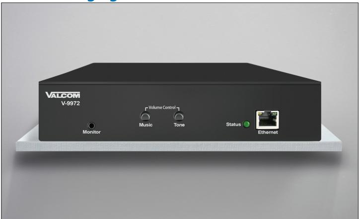
Valcom's V-9972 Universal Paging Interface is designed to provide access to paging systems from analog trunk or station inputs (FXO/FXS) and Session Initiation Protocol (SIP) voice over IP connections either through an on-premise PBX or Cloud PBX input. When paired with SIP connections the V-9972 supports Valcom handsfree page units for talkback paging and up to 150 Valcom one-way amplified speakers. The V-9972 connects multiple units for multi-zone paging.
