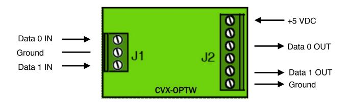
If voltage levels other than 5 volts are required at the output, then do not connect the internal pullup resistors. The outputs are now open collectors and will work with voltages from 5 to 24 VDC. Depending on the system, you may need pullup resistors to the higher voltage.
