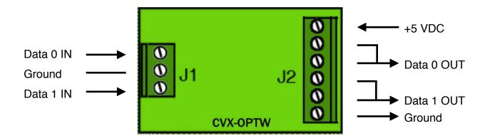
Previous versions of the CVX-OPTW had internal pullup resistors connected to the output ports. These pullup resistors were wired to the +5VDC supply. This newer version provides the option of connecting the pullup resistors in order to allow connection as a true open collector output.
