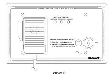
Figure 4 shows the SPRM front panel and the location of the LED's.
