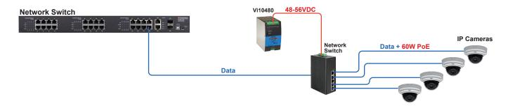
The Vi10480 can be used to power a wide variety high power PoE switches and Midspans.
