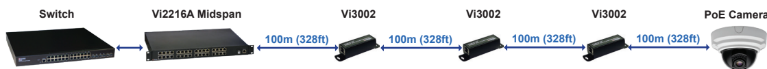
Multiple Vi3002 can be used to extend Ethernet and PoE. The maximum reach of PoE will be:
