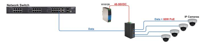
The Vi10120 can be used to power a wide variety high power PoE switches and Midspans.
