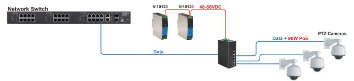
Multiple Vi10120 can share current to power a wide variety high PoE power PoE switches or Midspans. Also can be used as redundant power supply.
