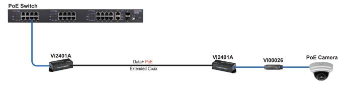
The Vi00026 requests maximum IEEE 803.2at PoE power from the PoE source to assure enough power for IP camera, extra power loss due to extended cable and Ethernet xtenders regardless of camera rated power level.
