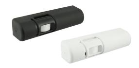
**SDC's MD-31D series motion sensors** are passive infrared detector specifically designed for request-to-exit applications. The coverage field is internally pointable. When angled 14 degrees down, coverage may be 5' x 6' at 7' feet high for 10' x 12' at 15' high. The MD-31D projects a wrap around "U" pattern down and away from the door to inhibit tampering.
