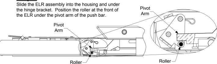
**Retrofit Installation Note:** 42" or 48" exit devices that have been modified to fit a 36" or smaller opening, may not have the required space to fit the standard E. L. R. assembly. Always verify the distance from the end of the touchpad to the end rail, and if necessary, consult with the factory for appropriate selection.
