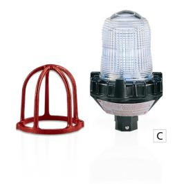
These models are hazardous location strobe lights that provide 60 high-intensity flashes per minute. This warning light is available in 24VDC with a 4-wire supervisable power circuit for fire alarm and suppression supervised control panels.
