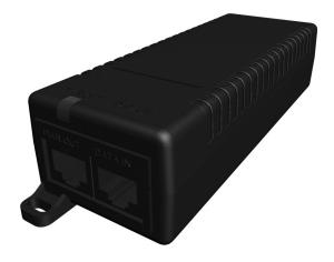
The POE130-AT Power over Ethernet (PoE) single-port midspan is designed to meet the demanding data rate and power requirements of IP cameras with high-quality streaming video capabilities. The PoE+ single-port midspan offers total output power of 30 W, and meets the IEEE802.3at standard for detection, connection, disconnection, and fault protection.
