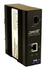
The SI-IES-111D-LRT is a (2) port unmanaged hardened PoE+ injector that adds up to 30 Watts of power from it's PoE+ Port onto a network segment. The gigabit speed SFP slot provides the ultimate flexibility by allowing fiber SFP uplink ports with varying communication distances.
