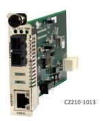
The ION C2210 is a media converter module that provides an interface between 10/100Base-TX ports and 100Base-FX ports, allowing users to integrate fiber optic cabling into 10/100 copper environments. Operating at Layer 2, the data link layer, this converter not only converts copper to fiber, it also provides rate conversion allowing legacy 10Base-T copper devices to connect to 100Base-FX fiber. The ION C2210 is a manageable device when installed in a managed ION chassis.
