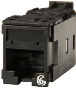
Clarity Cat 5E, CAT6 & CAT6A High Density Jack, ETL verified to TIA Category 5E, 6 & 6A component specification. Rear-loading, 180° exit, 8 position. Quick and easy lacing cap termination. Universal T568A/B wiring label. Center tuned to Clarity 5E patch cords for optimum performance.
