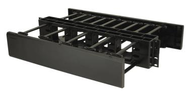
Legrand® horizontal cable managers are available in 1RU, 2RU, 3RU & 4RU sizes. Fingers begin 3/4" from the face of rack to provide bend limitation for cables, protecting cables, equipment and network performance. Included hinged cover mounts with six heavy duty clips allow them to be opened one handed without becoming "unhinged". Manufactured from UL94V-0 rated plastic. Available in Black and White.
