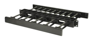
Legrand® horizontal cable managers are available in 1RU, 2RU, 3RU & 4RU sizes. Fingers begin 3/4" from the face of rack to provide bend limitation for cables, protecting cables, equipment and network performance. Included hinged cover mounts with six heavy duty clips allow them to be opened one handed without becoming "unhinged". Manufactured from UL94V-0 rated plastic. Available in Black and White.
