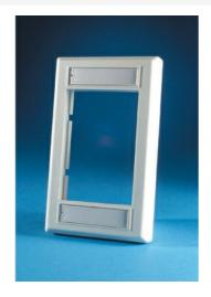
Legrand offers single and double gang Series II plastic Face Plates with a variety of module capacities to match your workstation applications. Series II plates offer recessed label fields, slotted screw holes to adjust alignment and are ruggedly constructed from high impact thermo-plastic 94V-0 rated to ensure long life.
