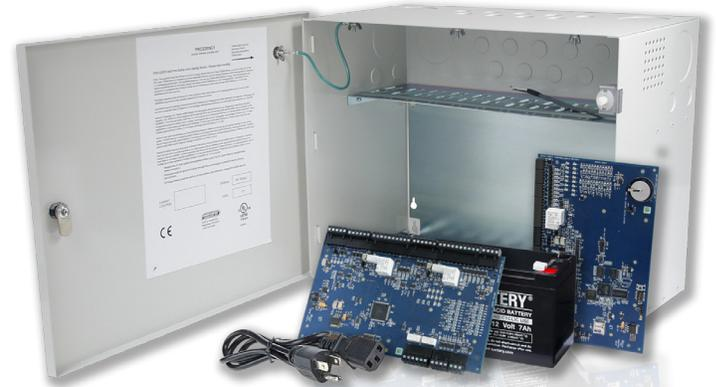
The PRO42IN interfaces provide 16 supervised alarm inputs and a dedicated power fail and panel tamper when tile mounted. An analog to digital converter samples the input values and the digitized result is filtered and processed. Filter parameters are configurable for each input point, resulting in the ability to specify a custom End-Of-Line (EOL) resistance value, sensitivity range and timing parameter.
