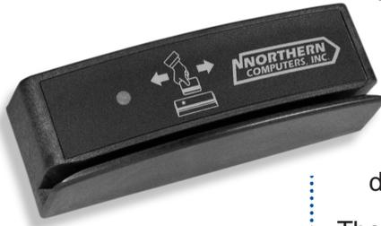
The BR-7 reader outputs in a Wiegand format and reads either 5 or 12 digit cards. It connects to Northern's N-1000-II, N-1000-III and N-1000-IV control panels.
