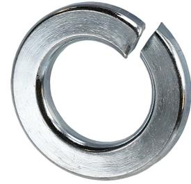
Split Lock Washers are manufactured with a trapezoidal cross section that deflects under load and can be used with or without a Hardened Flat Washer. They provide marginal resistance to vibration loosening and are ideal in applications where fasteners have a tendency to rotate or lose friction. Split Lock Washers are forged from hardened steel and zinc coated. They are covered by ASME B18.21.1.
