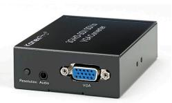
The KanexPro SDI to VGA Converter allows SDI, HD-SDI and 3G-SDI signals to be displayed on a VGA monitor or a projector ensuring high bit-rates up to 3 Gbps for faster signal transmission without loss in broadcasting quality signals. It provides signal re-clocking and equalization for longer length transmission up to 200 meters for HD signals and 300 meters for SD formats.
