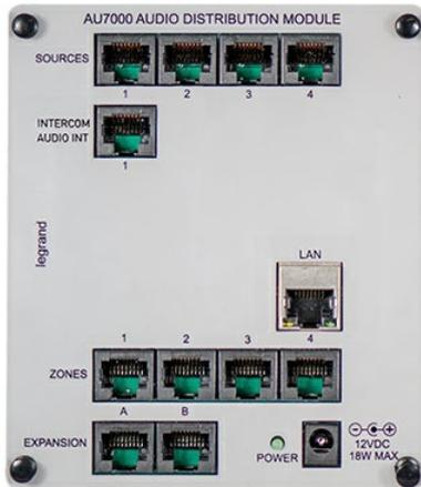
The Audio Distribution Module is used to connect up to four sources to the On-Q Digital Audio System and distribute those sources to four zone outputs. It can be expanded to accommodate up to sixteen sources and sixteen zones.
