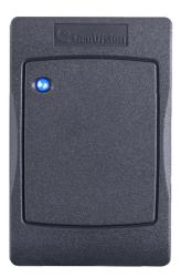
GV-SR1251 is a card reader designed to recognize access control cards. Featured with the Wiegand and RS-485 outputs, GV-SR1251 can be connected to any standard access control systems. GV-SR1251 comes with a weather sealed and IP66 compliant housing for outdoor use.
