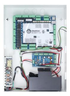
GV-AS8111 Kit is a cabinet containing a GV-AS8111, a power adapter board, a power supply and a casing for backup battery. The power supply provides power to GV-AS8111 Kit and up to 8 output devices (12V, 0.5A per device).
