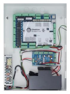
GV-AS4111 Kit is a cabinet containing a GV-AS4111, a power adapter board, a power supply and a casing for backup battery. The power supply provides power to GV-AS4111 Kit and up to 8 output devices (12V, 0.5A per device).
