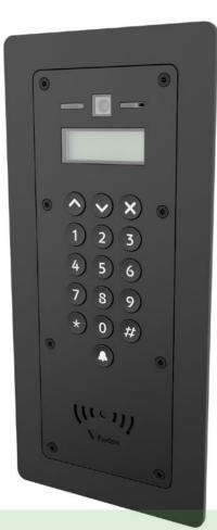
anel is a robust door entry panel incorporating entry and access control functions. It is powered er over Ethernet (PoE) and communicates with the ents of the system using IPv6, providing 'plug and ation. Each panel is associated with a Entry t which is the interface to the door hardware.
