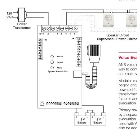
Return wires to evacuation panel for Class A operation.
