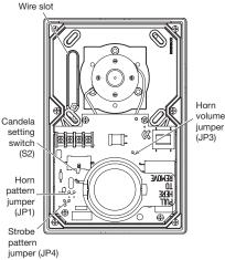
**Horn output:** Horns and horn-strobes are factory set for high dB output. Low dB output may be selected by cutting a jumper on the circuit board. This reduces the output by about 5 dB.
