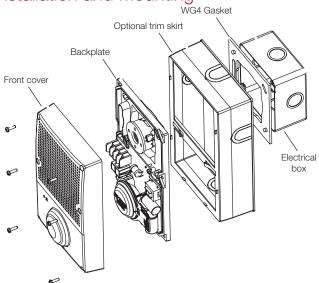
WG4 notification appliances are rated for outdoor use and are suitable for indoor or outdoor applications on walls or ceilings. For surface-mounting in outdoor or wet applications, appliances must be mounted to a 449 or 74347U electrical box. In dry conditions, they are compatible with standard 4-inch square by 1½-inch deep electrical boxes. When using the optional WG4WTS or WG4RTS trim skirt, a 449 or 4-inch square by 2-1/8" deep box must be used.
